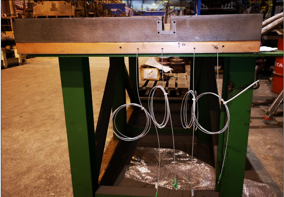
Fig. 3. Fibers installed on a horizontal axis in a copper broad face plate.
