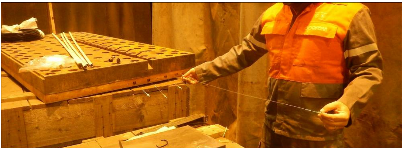
Fig.6 – Installation the fibers into the copper.
