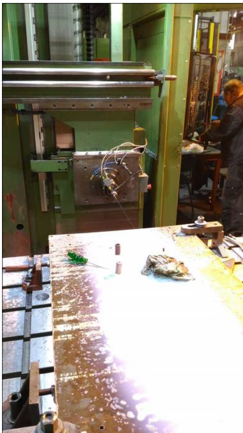
Fig.4 – Deep drilling holes
